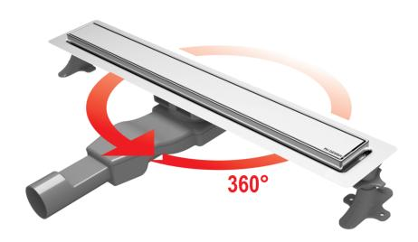
Flat stainless steel shower channel with 360° rotative PP drain. It is compatible with tiles from 15 to 28 mm and its feet are adjustable from 60 to 80 mm. Waterproofing fleece is included and perfectly adjustable on the stainless steel flange!
